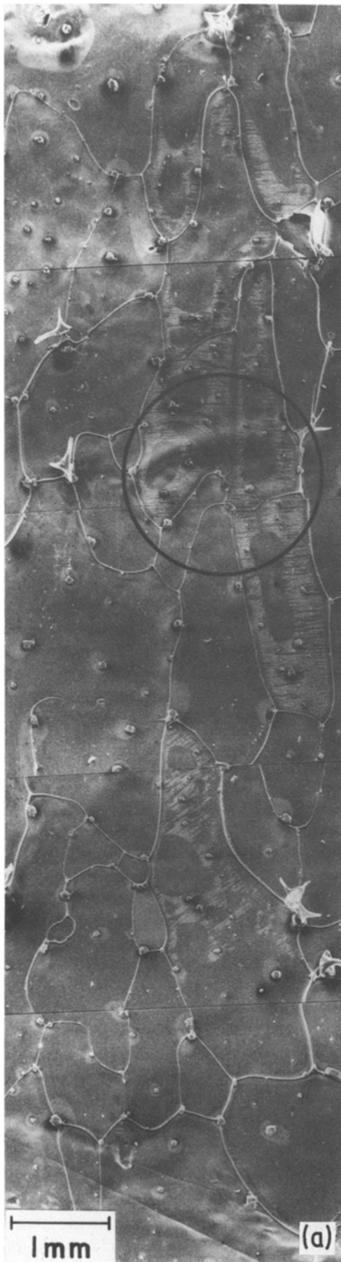
Figure 7 Scanning electron micrograph showing (a) replica of etched surface of vertical section, and (b) etch pits, encircled area in (a), elongated along [000 1] axes ( \longleftrightarrow ).
